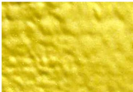
The PTS top coating shown below is an example of pinhole formation as a result of application over an improperly applied and cured sealer coating. The coating also exhibited very weak adhesion to the sealer layer.
